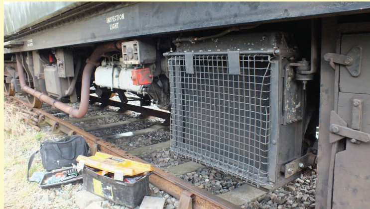
Replacement radiator fitted to M50455, 23/12/12
