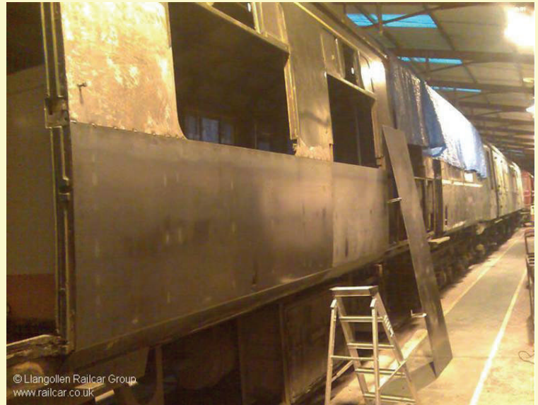
New metal welded into the drivers side middle saloon of 56456, 5/11/12 (Llangollen Railcar Group)
