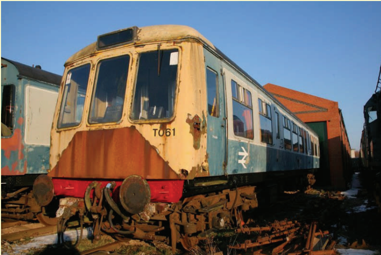
50645 before the cab end repairs were started at the Great Central Rly (North), 11/2/12 (DC-7C)
